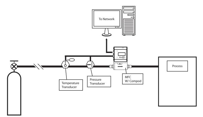
Temperature and pressure transducers are installed near the MFC. The 4-20mA signals from both are fed to the analog inputs of the Compod. The Compod communicates via its RS485 MODBUS output to the network. When the master control system needs to know information on this process, it sends a request to the Compod, which then reports the flow, temperature and pressure. The control system can also regulate the flow by sending setpoint commands to the MFC via the Compod.
