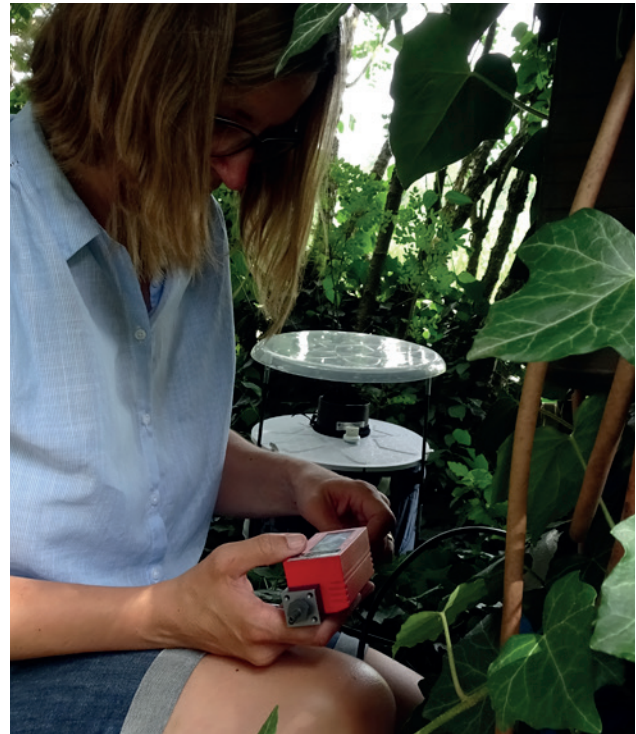
A Biogents employee checks the CO 2 gas flow with the help of a red-y compact
