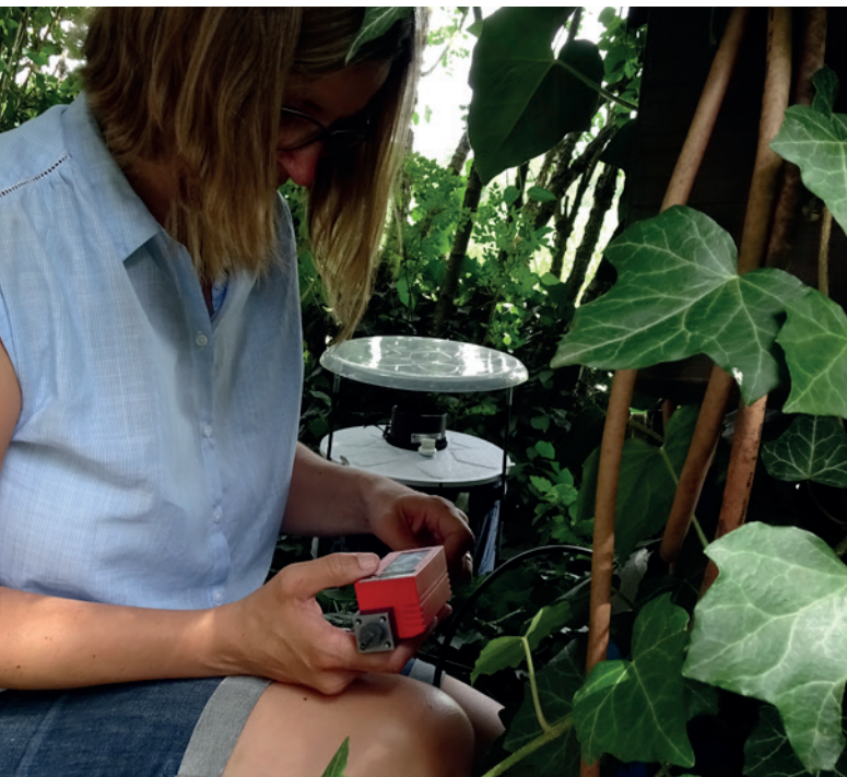
Fig. 4 A Biogents employee checks the CO 2 gas flow with the help of a red-y compact
