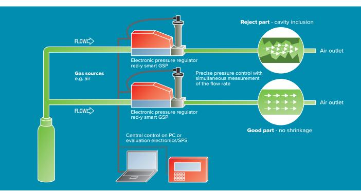
Fig. 1 Functional process scheme on the inspection of engine components for blowholes
