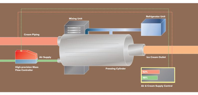
Fig. 1 Functional process scheme of ice cream manufacturing
