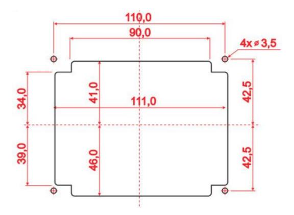
The four pre installed distance pins are planned for a front wall thickness of 2 mm und should be adjusted to the actual wall thickness.
