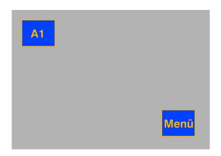
In the "MFC-Control" operating mode each button stands for a single registered MFC (Mass Flow Controller), MFM (Mass Flow Measurement) or GPC (Gas Pressure Controller). The number after the "A" is identical to the address of the MFC, MFM or GPC. Each connected device must have a unique address in the system via which it can be addressed by the PCU-10. The micro-controller
