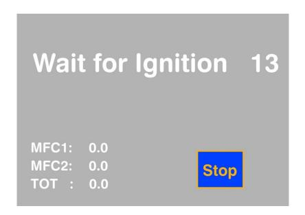
The big "Start Oven" button opens both solenoid valves and sets both MFCs to a specified setpoint. This setpoint is the one which arises from the parameterization of the burner controller for the ignition.
