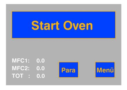
The Burner Controller is used for the controlled ignition of an oven and its monitoring after ignition. First both MFCs and both solenoid valves are closed. The actual values of both MFCs are displayed in the bottom left corner of the screen.
