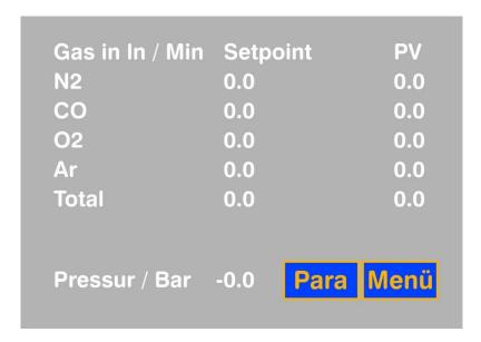
The names of the gases (automatically read out from the MFCs) appear underneath the column headings as well as the setpoints and PVs (process value) for the 2-4 MFCs, which form the mixer.
