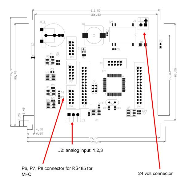
Connector sockets on the display pcb:
