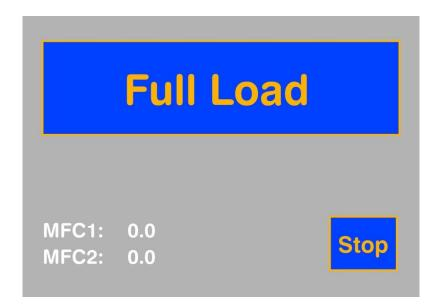
With this the Burner Controller is informing the user that everything is okay and that you can switch to the second gas mixture by pressing the button. *The second gas mixture is the one which results from the parameterization of the burner controller for the full load range.* After shifting to the second mixture the display changes to:
