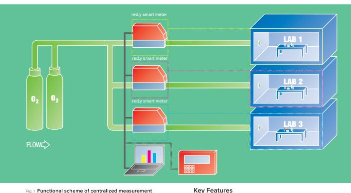
Fig. 1 Functional scheme of centralized measurement
